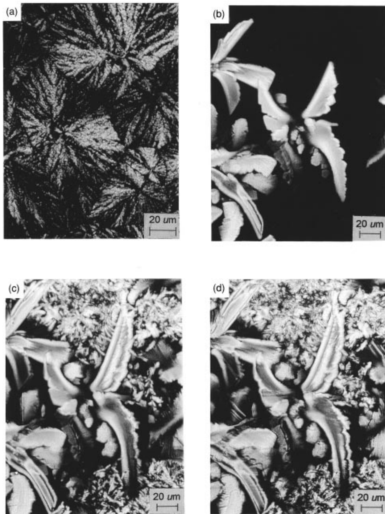
Figure 6. Optical micrographs of sheared C12HPC. (a) Slowly cooled from the isotropic state to 25 °C, 400×; (b) reheated sample a to isotropic state followed by step-cooled to 99 °C, 300×; (c) step-cooled sample b to 90 °C, 300×; (d) step-cooled sample c to 25 °C, 300× (see text for step cooling).
